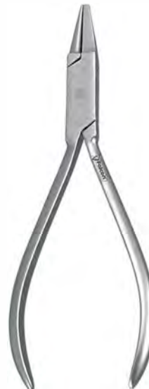
DO.610.300 Falcon Light wire bending and loop forming pliers Kleszcze do zaginania drutu i formowania pętli ● 0.36 mm to 0.50 mm (.012" to .020") ■ Max. 0.41 mm x 0.56 mm (.016" x .022")
